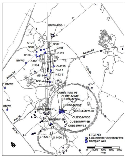
Figure 6.4-2 - Groundwater monitoring well locations in 2014. Sampled wells represented by labeled, filled circles. Wells used only for groundwater elevations represented by half-open circles. (Original DUSAF projection.)
